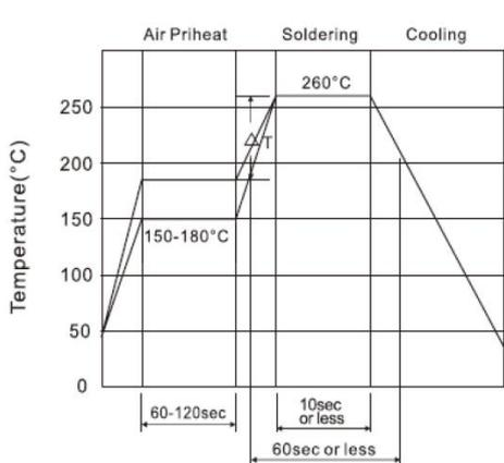
The graph shows a temperature profile for reflow soldering. The y-axis is Temperature (°C) from 0 to 250. The x-axis is time. The profile is divided into three stages: Air Preheat (60-120sec), Soldering (10sec or less), and Cooling (60sec or less). The temperature rises to 150-180°C during preheat, then to 260°C during soldering. A temperature difference ΔT is indicated between the preheat and soldering stages.
